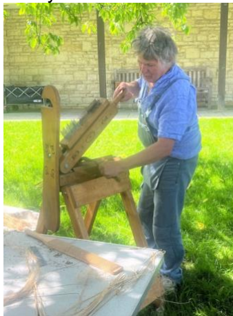
Using a flax break. Hackle on top and scutching knife on table
